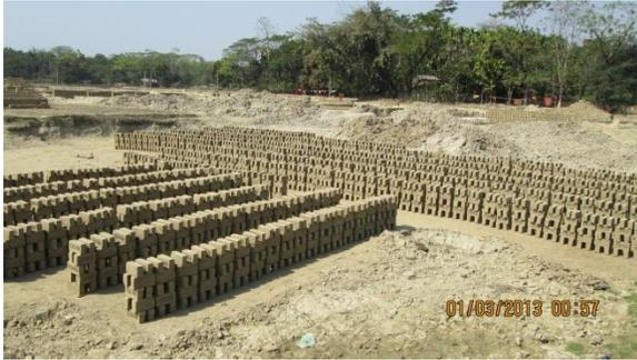
The Columbia Electronic Encyclopaedia (2004): A brick is a block of ceramic material used in masonry construction, laid using mortar. Brick is made by pressing clay into blocks and firing them to the requisite hardness in a kiln. Bricks in their most primitive form were not fired but were hardened by being dried in the sun.
